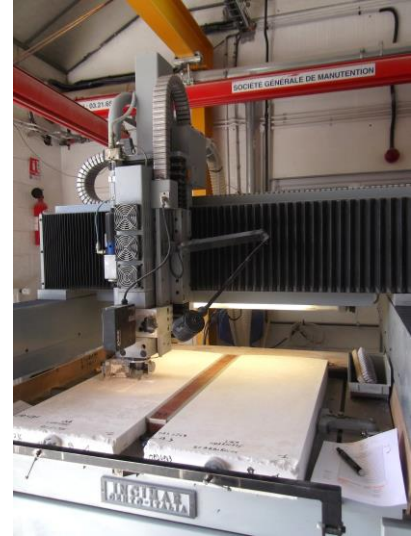
The machines on which new and replacement headstones are engraved.
