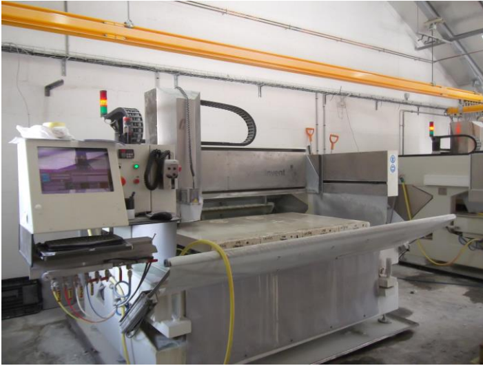
The machines on which new and replacement headstones are engraved.
